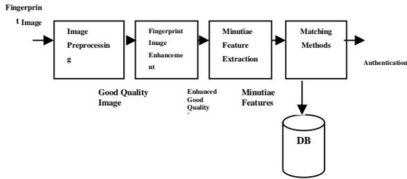
Figure 4 Fundamental Structure of the Fingerprint Verification system
